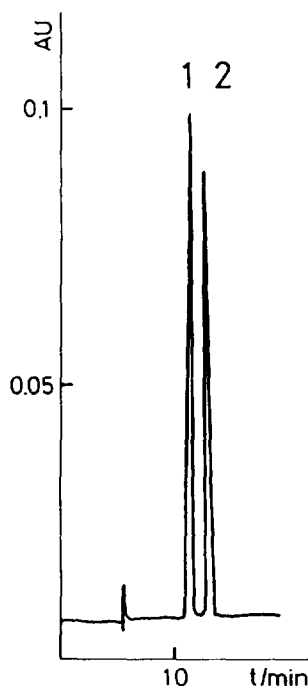
Fig. 2. Chromatogram of D,L-threo- and D,L-erythro- \beta -methylphenylalanine. Column, Vydac 218TP54 C 18 ; flow-rate, 1.5 ml/min; mobile phase, 0.2% acetonitrile in water; detection at 210 nm. Peaks, 1 = D,L-threo-; 2 = D,L-erythro- \beta -MePhe.
